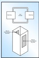
LINE POSTS: Used where two sections of fence meet and are running in a straight line. Some angle variation possible.
