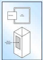
END / GATE POSTS: Used where a fence line starts and ends including when a gate will be installed on any remaining side.
