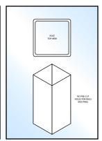
BLANK POSTS: Used when no fence is to be attached as would be the case for a gate at the end of a fence line.
